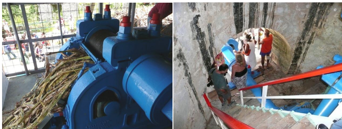
Figure 85. Cane crushing rollers within Morgan Lewis Mill and interior mill access ( Source: Barbados National Trust, 2013).
