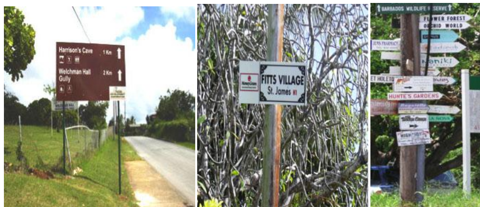
Figure G9. Place of interest sign (left), confirmatory/place name sign (middle), and typical signage clutter (right).
